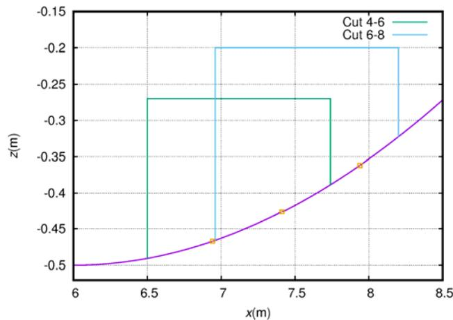
**Figure 7** Position of the two cuts for the passenger aircraft fuselage (S1D, green; S1E, cyan) on the middle x-z plane. Note that different scales are used for the vertical and horizontal axes
