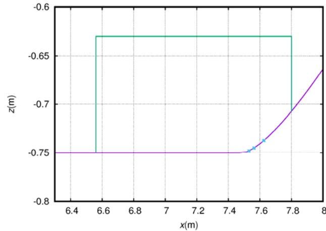
**Figure 8** Position of the cut for the transport aircraft with circular cross section (S2): note that different scales are used for the vertical and horizontal axes
