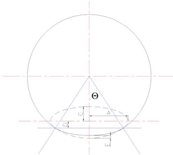
**Figure 4** Sketch defining the circular-elliptical cross section
