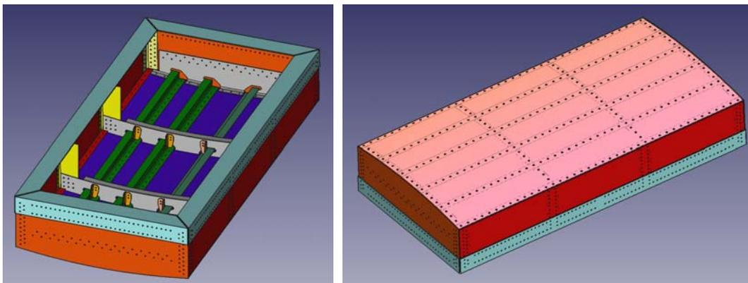
**Figure 11** Top and bottom views of the CAD model of the aircraft-like structure
