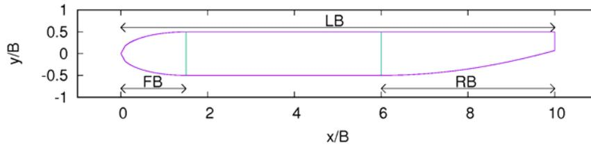
**Figure 1** Parameterization of the fuselage shapes
